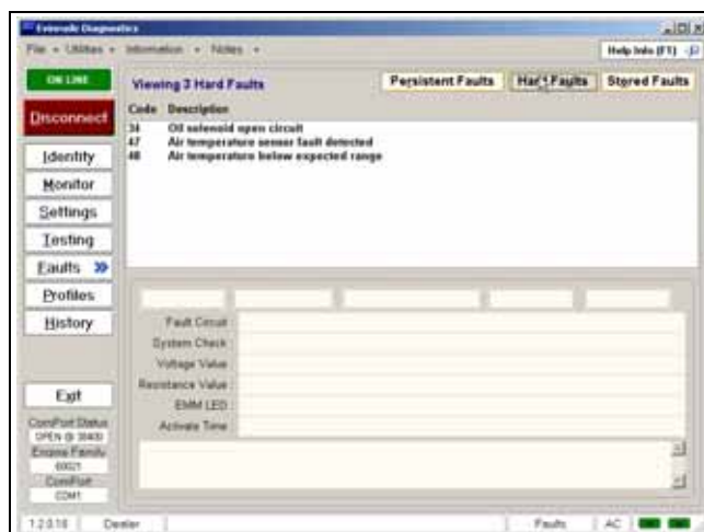
Stored Faults Review Screen
