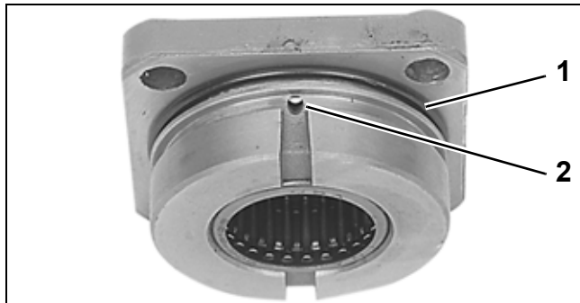
1. O-ring (top groove) 2. Oil passage
