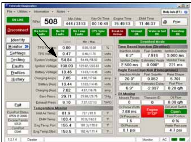
Engine Monitor Screen, System Voltage
