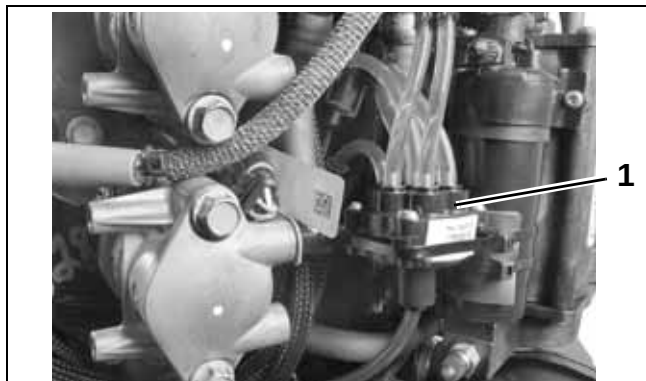
1. Rear oil manifold
