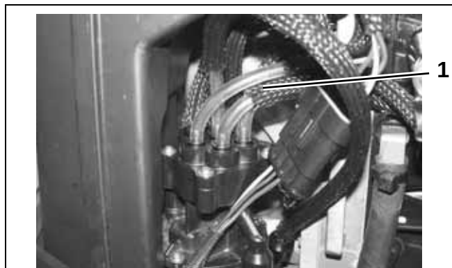
1. Oil distribution hoses (7)
