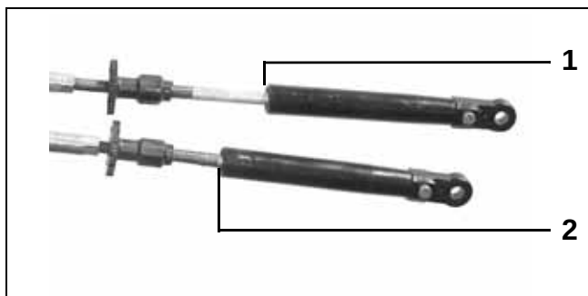
1. Shift cable casing guide extended to midpoint 2. Throttle cable casing guide retracted
