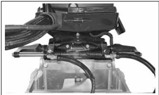
TYPICAL Manual Hydraulic Steering 004948
