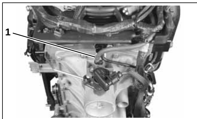
1. Vent hose connection to intake
