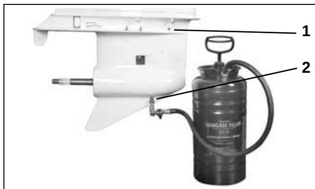
1. Lubricant level plug 2. Lubricant drain/fill plug
