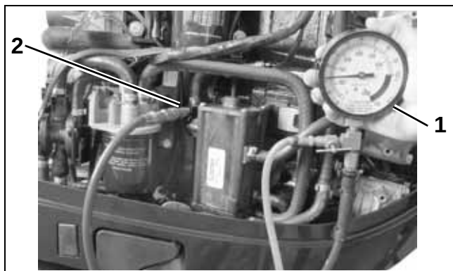
1. Fuel pressure gauge 2. Test fitting
