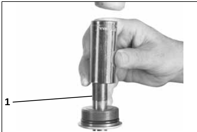
1. Tilt Cylinder Seal Protector P/N 326005
