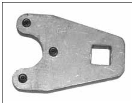
Tilt cylinder end cap remover 005340 P/N 352932, for single-piston tilt systems
