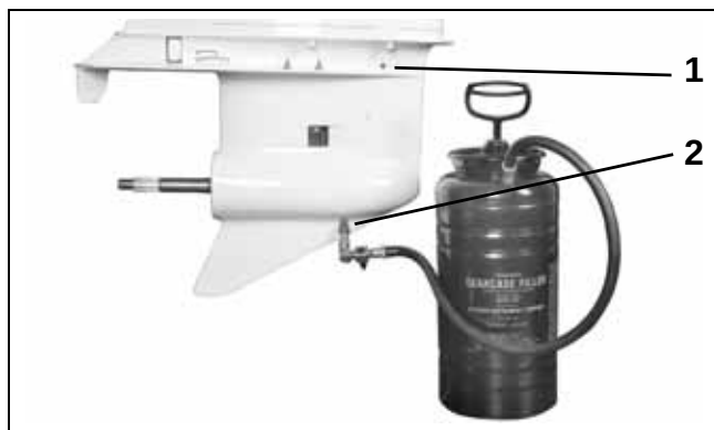
1. Lubricant level plug 2. Lubricant drain/fill plug
