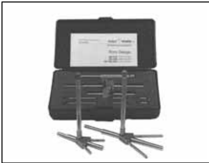
Cylinder bore gauge P/N 771310 45303
