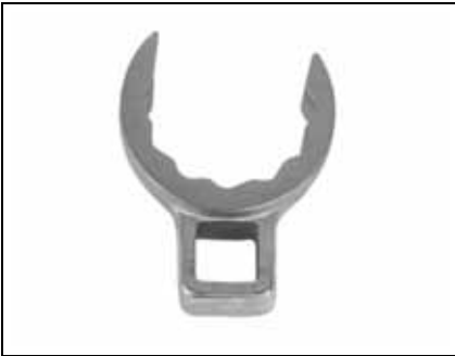
Tilt tube nut wrench P/N 342680 46879
