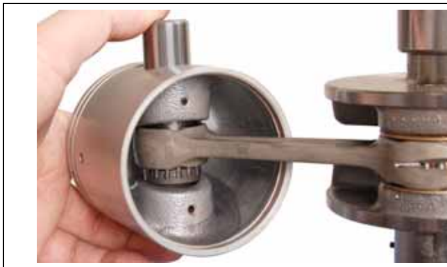
1. Gap of retaining ring 2. Notch in piston
