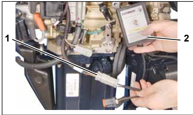
1. Engine harness key switch connector 2. Power supply tool
