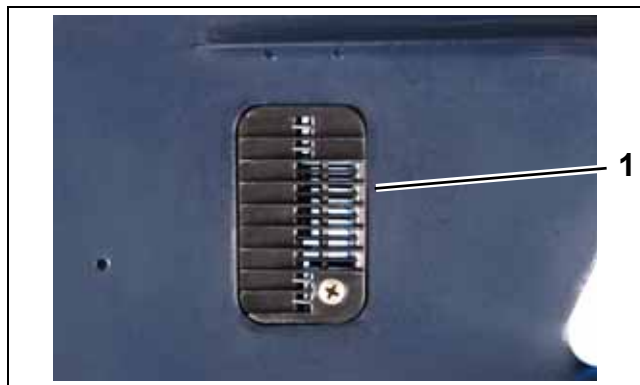
1. Water intake screen
