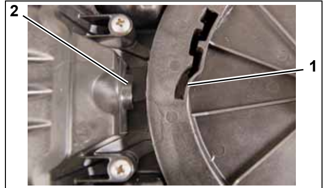
1. Rope channel 2. Rope guide
