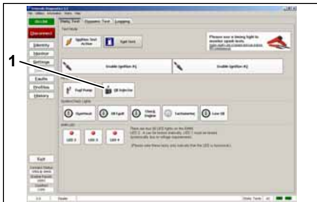
Static Tests Screen 1. Oil injector test button
