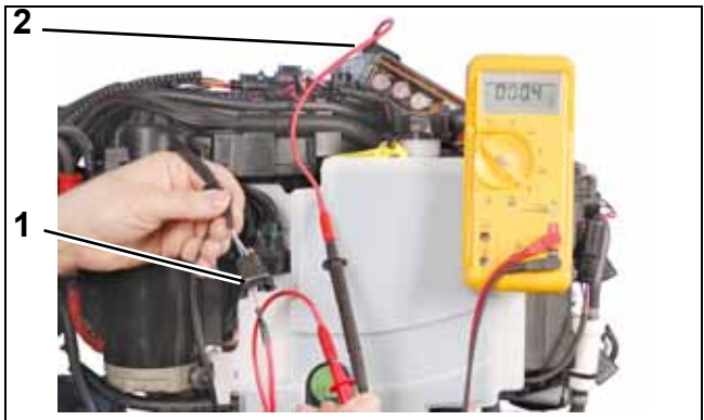
1. Oil injection pump connector pin A 2. EMM connector pin 2 007328
