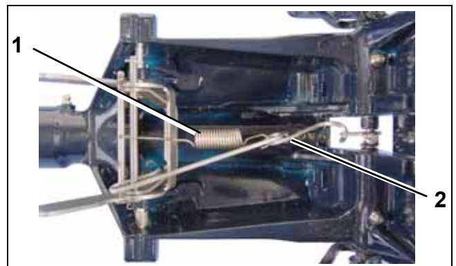
1. Spring 007615 2. Reverse lock release rod
