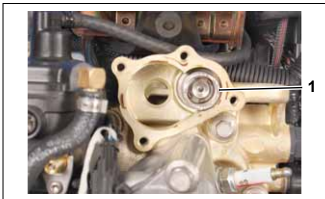
1. Spring, thermostat and gasket
