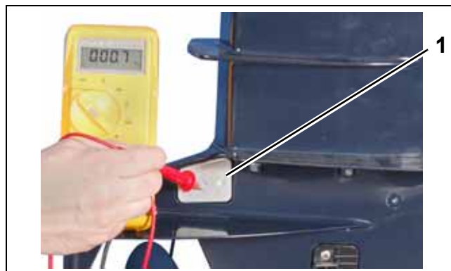
1. Meter lead to anode
