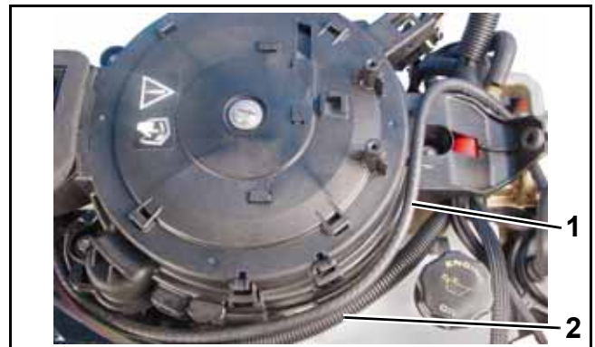
1. Vapor separator vent hose 2. Wiring
