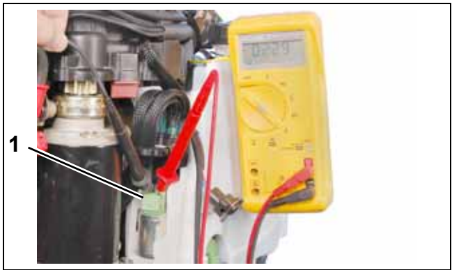
1. Oil injection pump connector 007329
