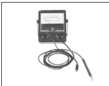
Peak reading voltmeter 49799 P/N 507972
