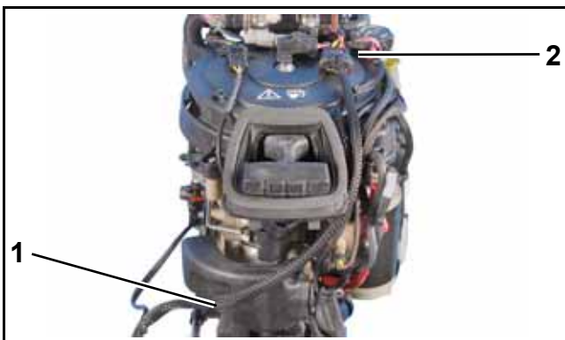
1. Wire routing 2. Retainer 007474
