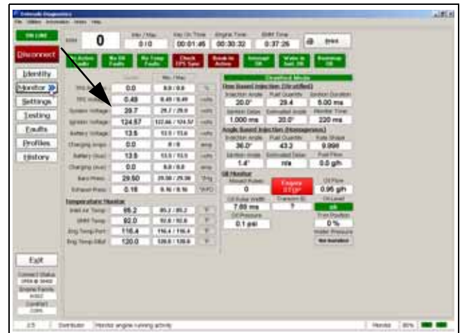
Engine Monitor Screen, System Voltage
