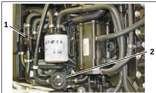
1. Front mounted pump 2. Side mounted pump
