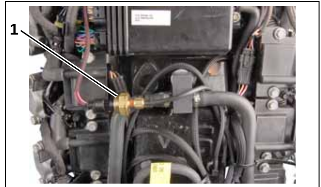
1. Water pressure transducer 008131
