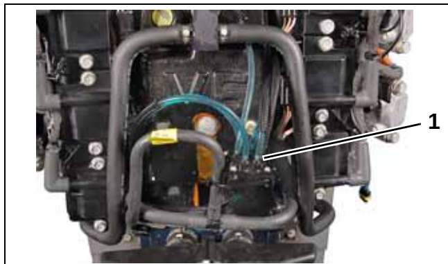
1. Rear oil manifold – 3.4 L models
