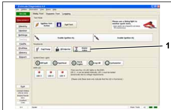
Static Tests Screen 1. Water valve test button
