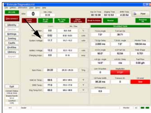
Monitor Screen, System voltage
