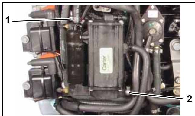
1. Fuel supply manifold 2. Fuel return manifold
