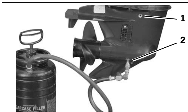
1. Lubricant level plug 2. Lubricant drain/fill plug
