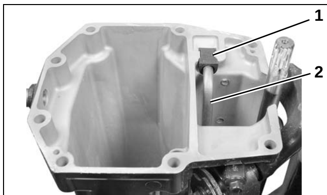
1. Water tube 2. Grommet
