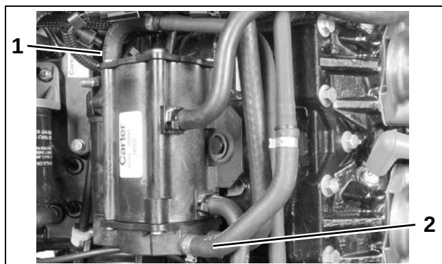
1. Fuel supply manifold 2. Fuel return manifold
