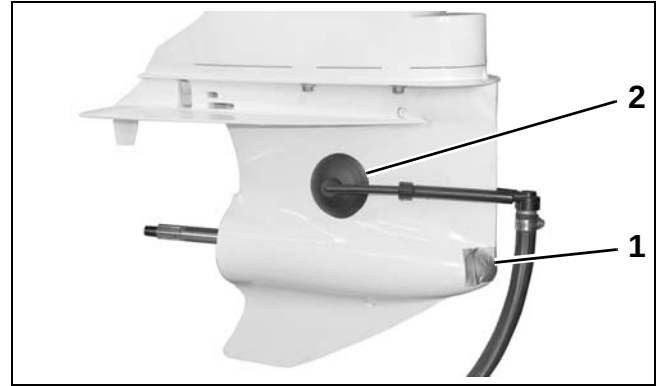
M2-Type Gearcase 1. Water-proof tape 2. Flushing adapter
