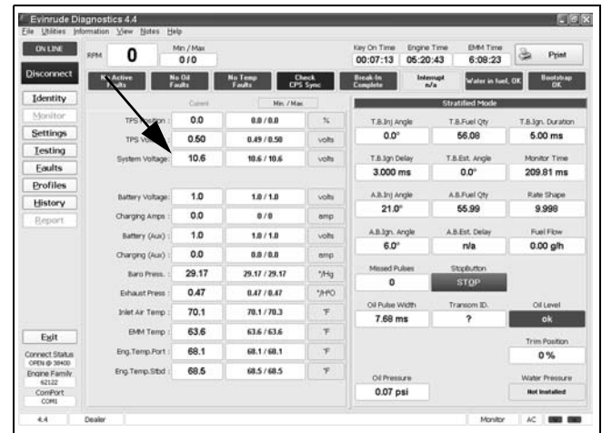
Engine Monitor Screen, System Voltage
