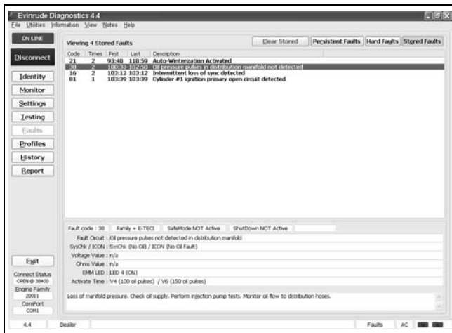
Stored Faults Review Screen
