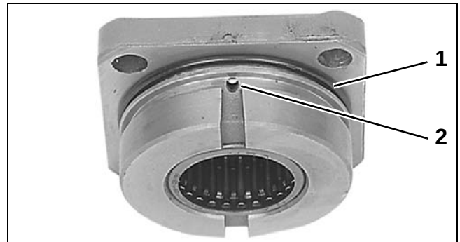
1. O-ring (top groove) 2. Oil passage
