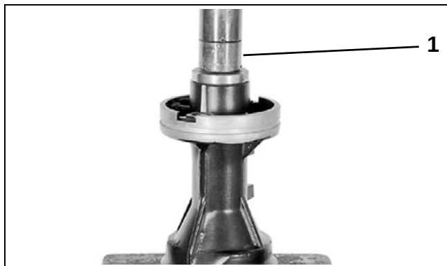
Rear Bearing 1. Bearing installation tool
