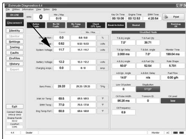
Monitor Screen, System voltage
