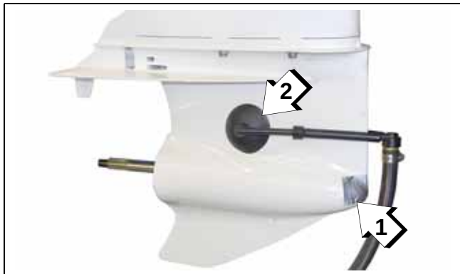
M2-Type Gearcase 1. Water-proof tape 2. Flushing adapter
