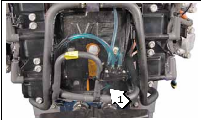
1. Oil to rear manifold
