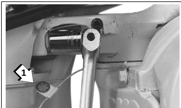
1. Ground lead (removed)
