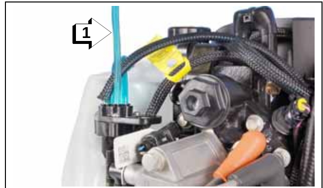
1. Temporarily installed length of oil hose
