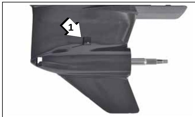
1. Water intake screen
