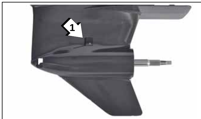
1. Water intake screen
