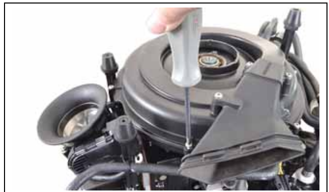
Air Duct (Typical)
