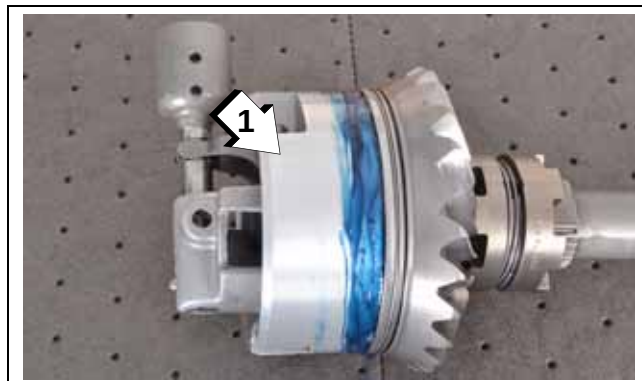
1. Triple Guard grease applied to leading edge of shifter housing
