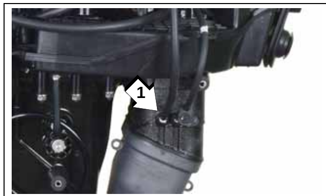
1. Exhaust pressure fitting
