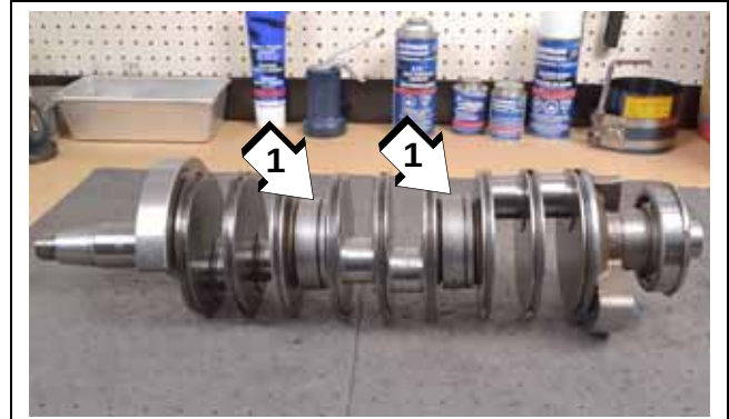
1. Split sleeve ring grooves toward driveshaft
