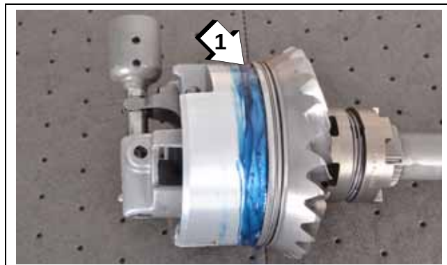
1. Triple Guard grease applied to rear edge of shifter housing
