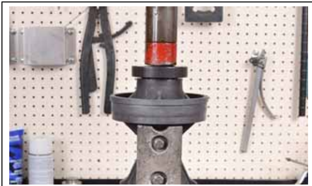
Rear Bearing 1. Bearing installation tool
