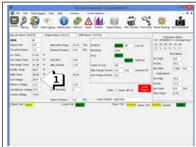
Engine Monitor Screen, System Voltage Display
