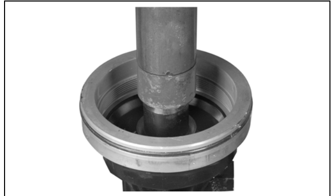
Front Bearing 1. Bearing installation tool
