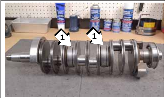
1. Split sleeve ring grooves toward driveshaft
