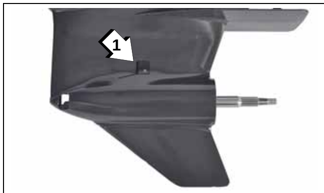
1. Water intake screen
