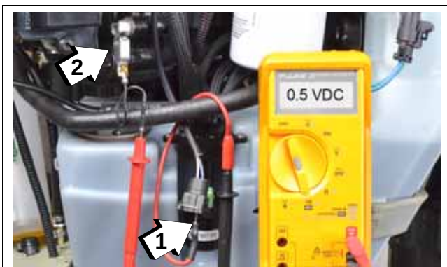
Oil Pump Connector 1. Black meter lead to pin B, blue or blue/orange wire 2. Red meter lead to engine ground
