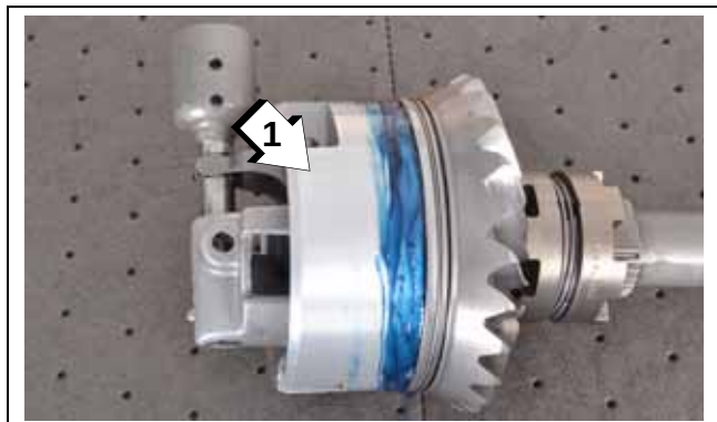
1. Triple Guard grease applied to leading edge of shifter housing
