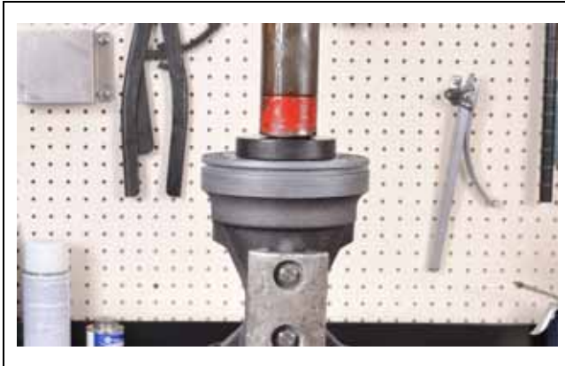
Front Bearing 1. Bearing installation tool
