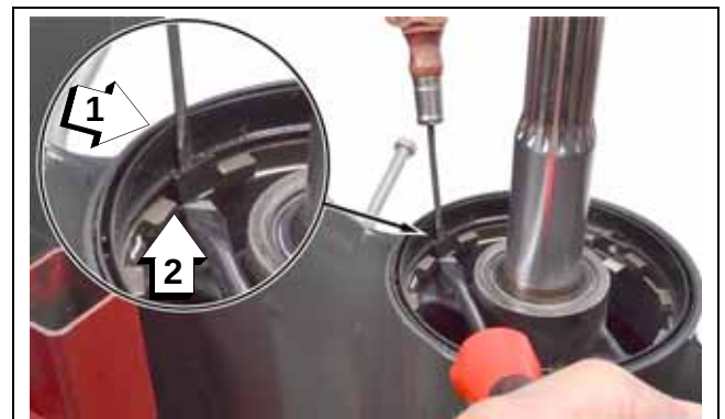
1. Pry tab inward 2. Pry ventilation ring up
