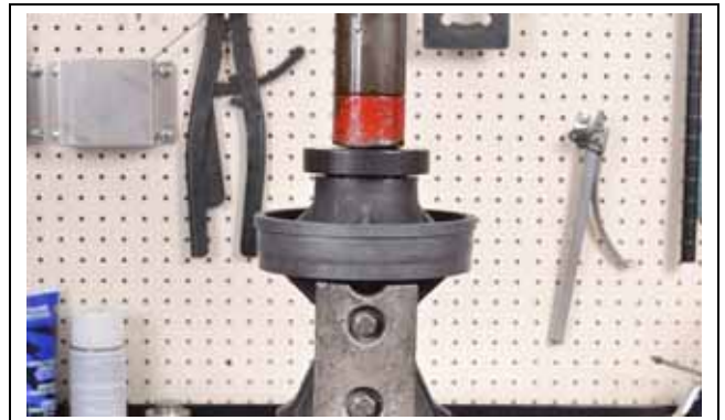
Rear Bearing 1. Bearing installation tool
