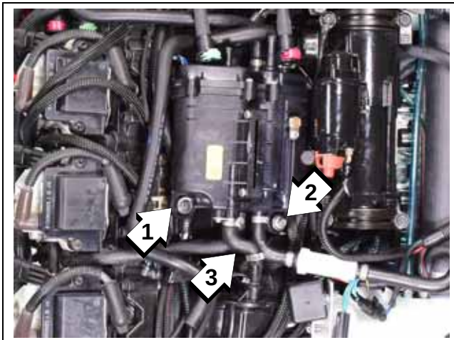
1. Spacer, washer and M6 x 50 screw 0106700 2. Washer and M6 x 25 screw 3. Short fuel hose with 17 mm clamp
