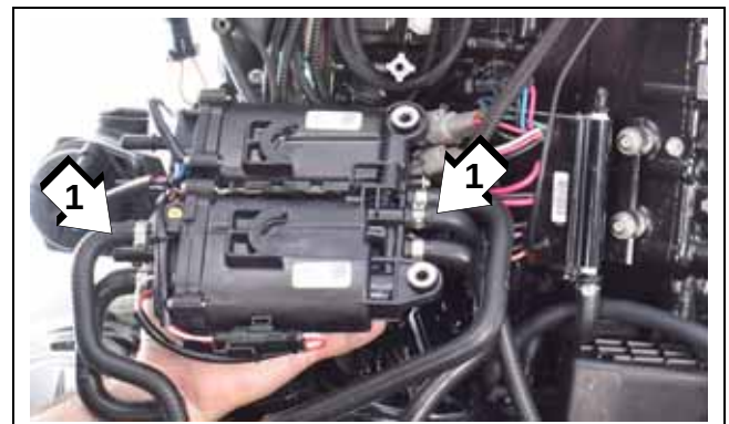
1. Cooling water hoses
