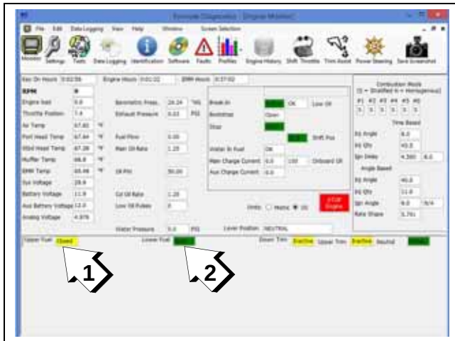
Monitor Screen 1. Upper fuel micro switch 2. Lower fuel micro switch
