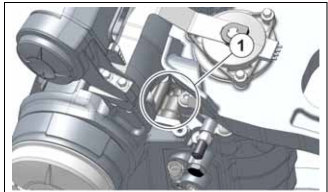
1. Wiring pass-through area
