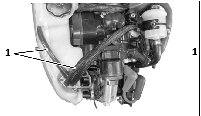
1. Oil distribution hoses
