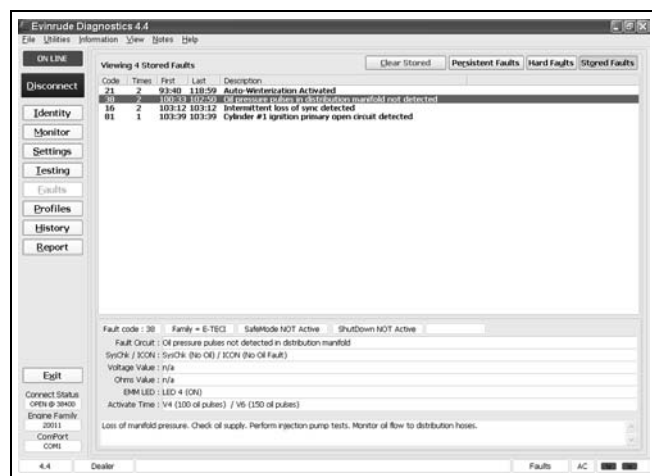
Stored Faults Review Screen
