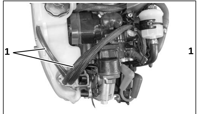
1. Oil distribution hoses
