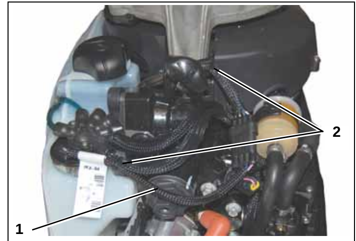
1. Oil pump wire harness 2. Tie straps
