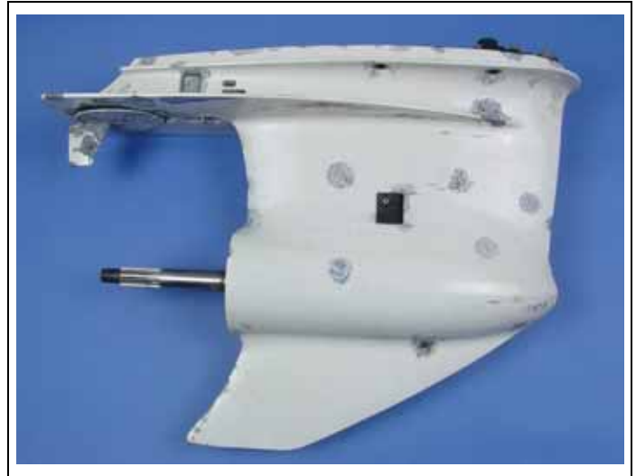
Stray current corrosion
