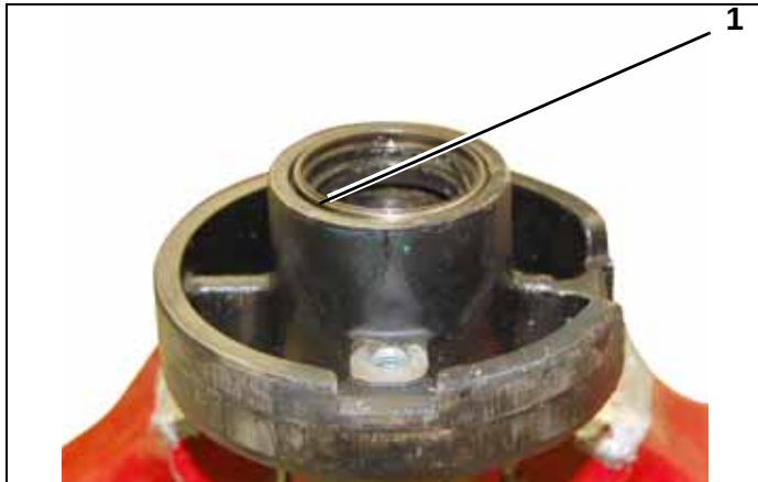
2. Propeller shaft seal pushed out
