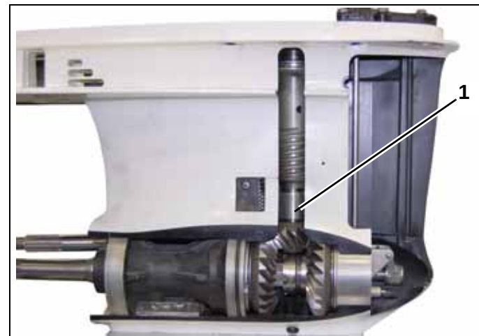
1. Pinion bearing, P/N 5007751 has increased taper
