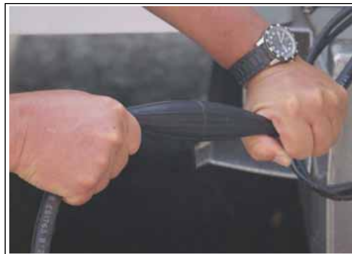
Damaged fuel primer bulb
