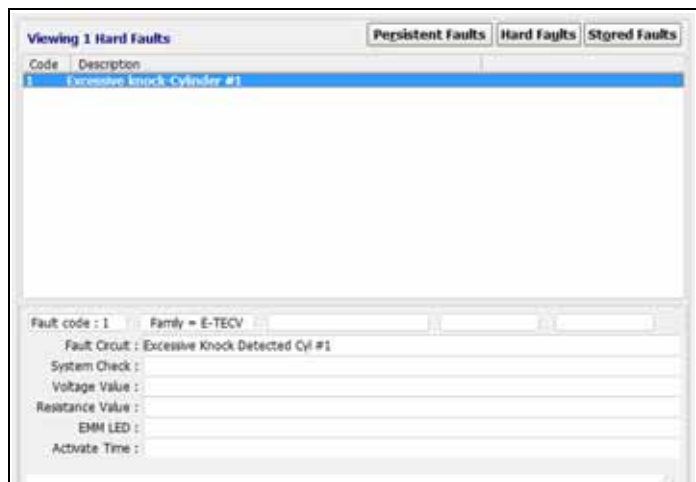
Code 1; Excessive knock detected cylinder #1
