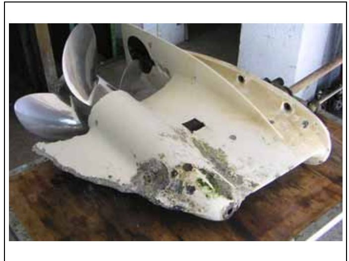
Stray current corrosion
