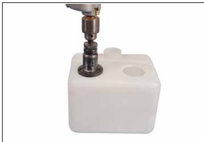
Use 1-1/2 in (38 mm) hole saw to enlarge tank for oil level converter
