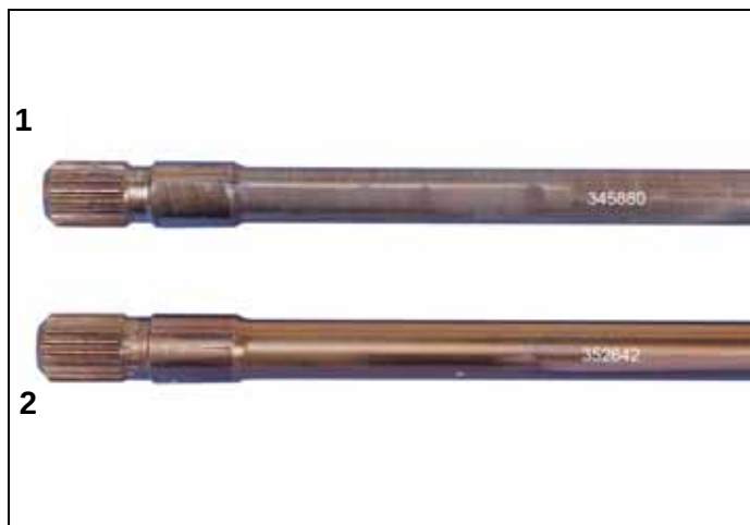
Part number stamped on driveshafts
