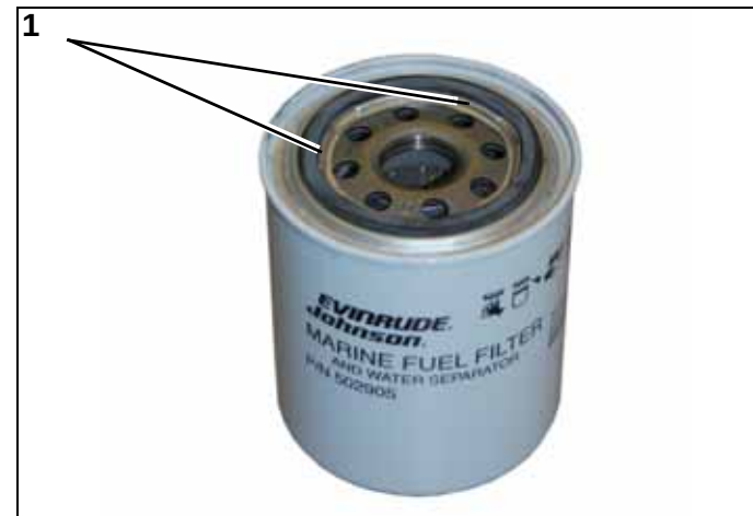
1. The seals on Evinrude / Johnson Genuine fuel filters are crimped
