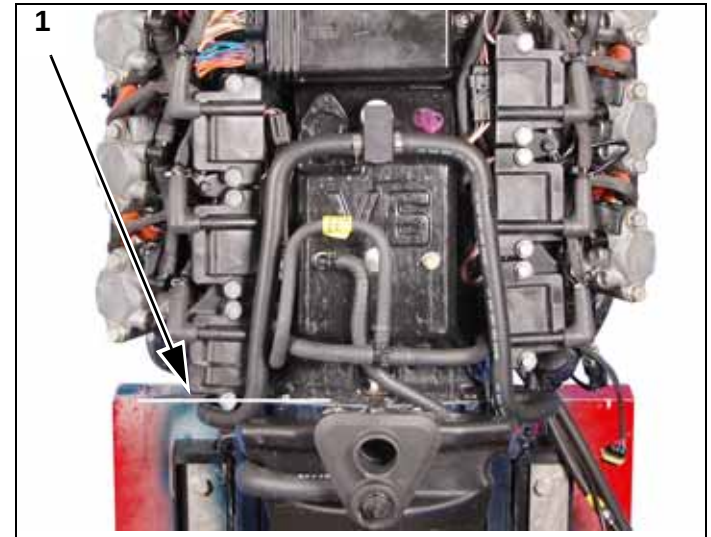
1. Ignition coil mounting, 90° V6 models
