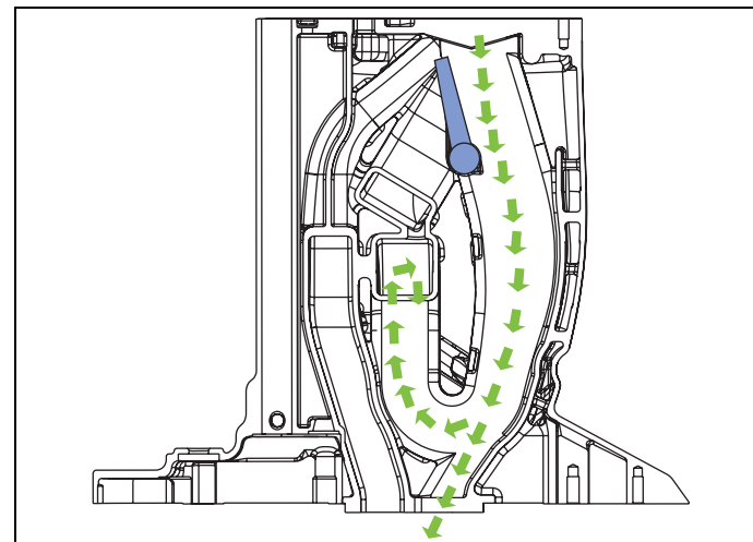
Exhaust valve, low speed position (cut-away view)
