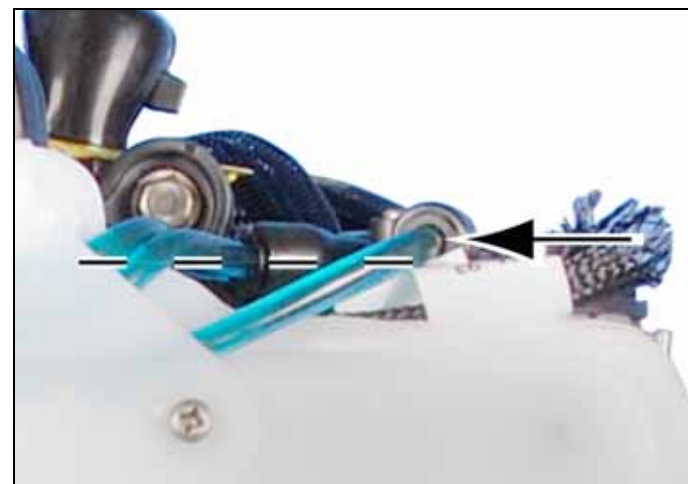
Oil port is physically located higher on the oil manifold
