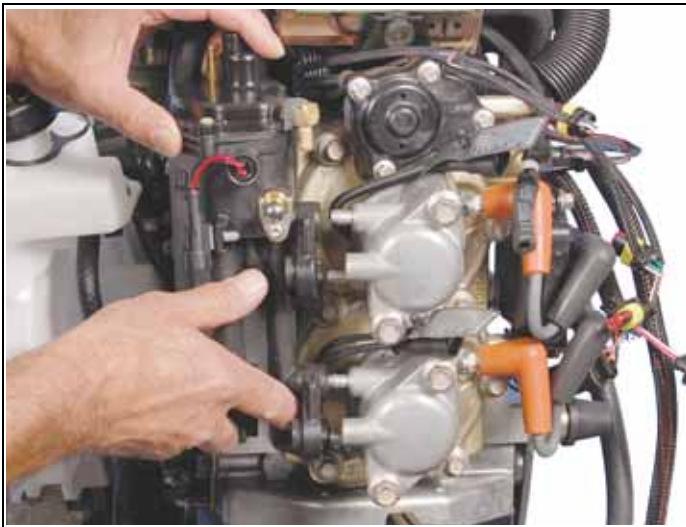
Installing vapor separator to fuel injectors
