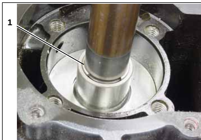
Driveshaft - driveshaft bearing housing removed
