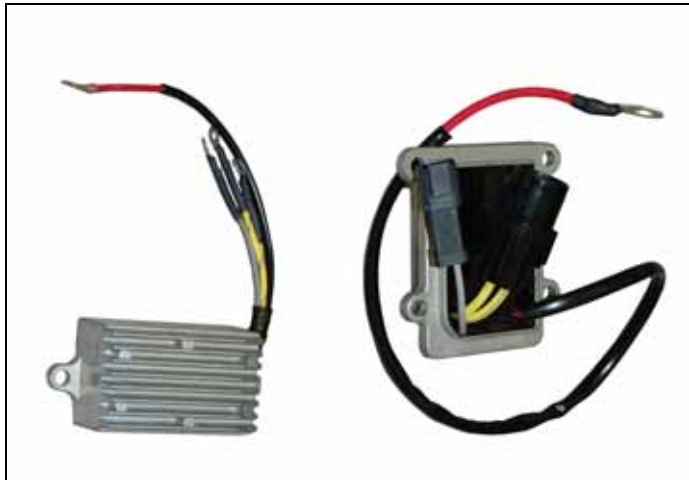
Improved rectifier/regulators do NOT have a purple lead
