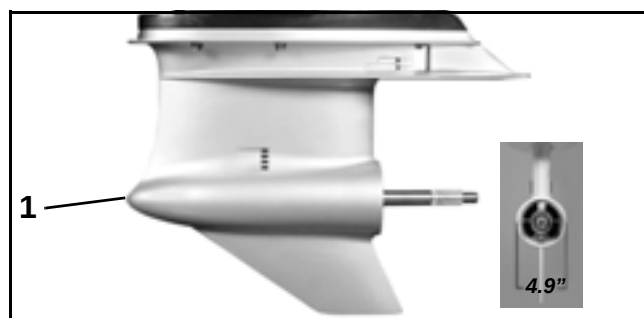
"L"-Type Gearcase (2001 and newer FHL models)
