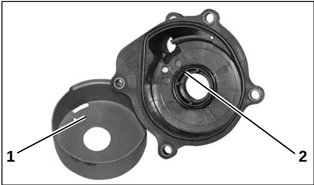
1. Vent hole in impeller cup 2. Impeller housing vent
