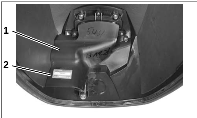
Inside of Upper Engine Cover 1. Baffle 2. EPA label
