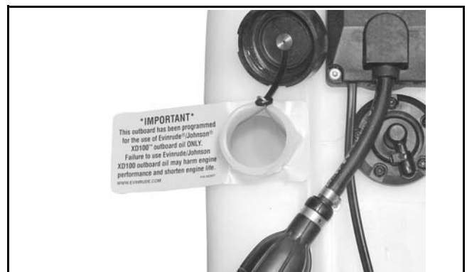
Remote Oil tank
